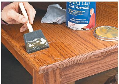
A thick, gel varnish brushes (or wipes) on easily. Then you can just wipe off the excess for a smooth, even look. Plus, buildup goes quickly since the finish dries fast.
