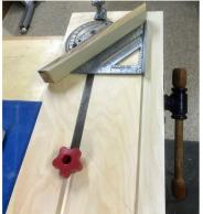
sure, the Craftsman miter gauge can be moved out of adjustment in the planing process if you only hand tighten the locking knob. I use some large pliers to crank it down the so the adjustment doesn't move. I am sure the \$\$\$
