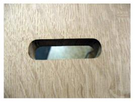
Step 4 – square the corners in the usual way with a chisel.
