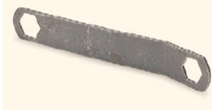
Bending the wrench isn't difficult. I just clamped the end in a vise and applied a little force. And I've definitely seen a good return on this small investment.
