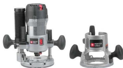
2-1/4 HP (Maximum Motor HP) Multi-Base Router Kit 893PK - The 893PK includes Router motor, Fixed base, Plunge Base, 1/4" & 1/2" collets, Sub-Base Centering Gauge, Collet wrench, Carrying Case, Operating manual.
