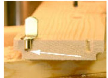
The holes should be slightly deeper than the length of the pin to insure a flush fit.
