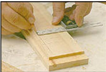
A 6" combination square is perfect for laying out the pin hole locations. Here the blade is used to trace the vertical lines onto the cabinet side piece.
