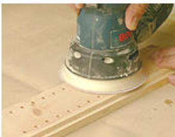
Sanding the interior surfaces is easier now anyway so sand the layout lines away in the process.
