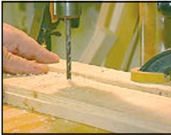
Even a small drill press makes drilling the holes accurately fast and simple.
